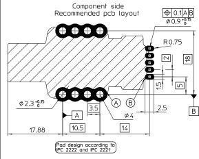
(Layout example with 4 jumpers in parallel)
