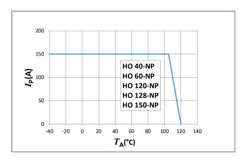
Important notice: whatever the usage and/or application, the transducer jumper temperature shall not go above the maximum rating of 120 °C as stated in page 3 of this datasheet.
