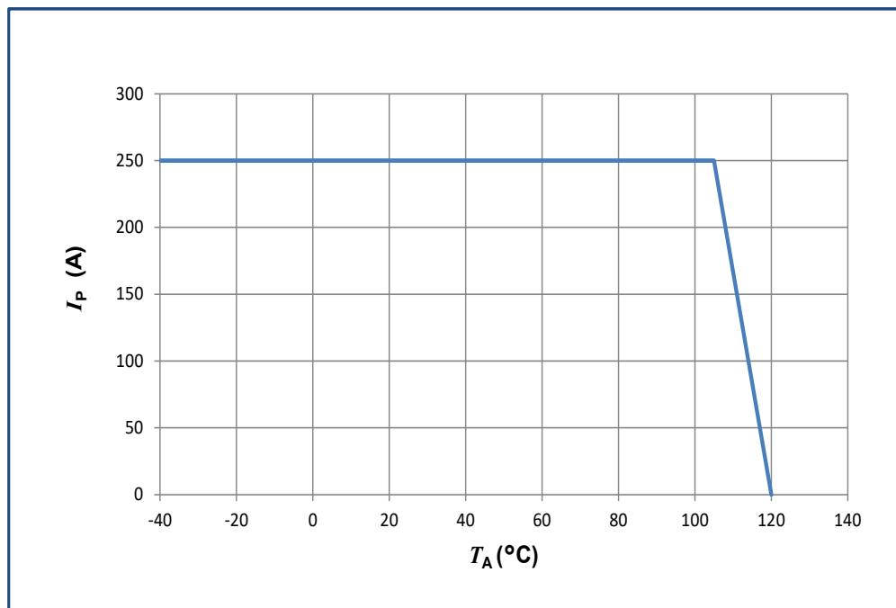
Important notice: whatever the usage and/or application, the transducer primary bar / jumper temperature shall not go above the maximum rating of 120 °C as stated in page 2 of this datasheet.
