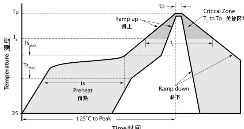
Recommended reflow methods: IR, hot air oven,  $\text{N}_2$  environment for lead-free. 推荐回流焊方法: 红外线, 热空气, 氮气, 无铅。
